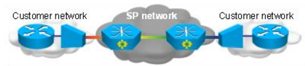
Figure 9: Fiber interconnection by using one or a few wavelengths at a service provider
