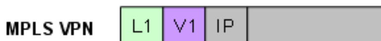
Figure 1: MPLS VPN label encapsulation. Label L1 is the path label (provided by LDP), label V1 is the VPN label (provided by BGP)
