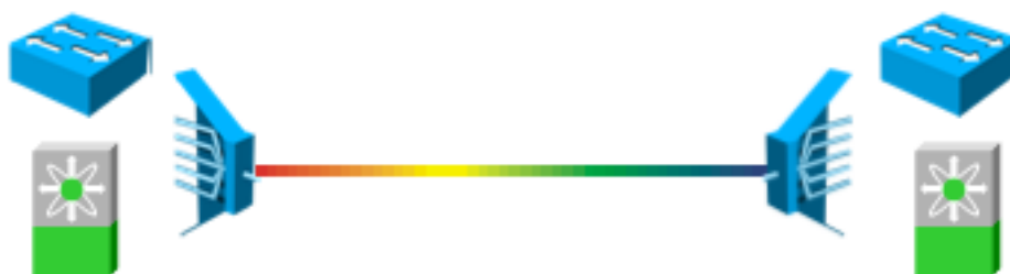
Figure 8: Dark Fiber interconnection using CWDM or DWDM. Multiple channels can be set up, i.e. one for Gigabit Ethernet, one for Fibre Channel
